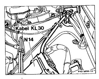
Disconnect cable terminal 30 for preheating relay at cable connector X4 on fuse box and relay box, cut off connector lug.
