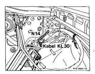
Disconnect cable terminal 30 for preheating relay at cable connection X4 on fuse and relay box, cut-off connector lug.
