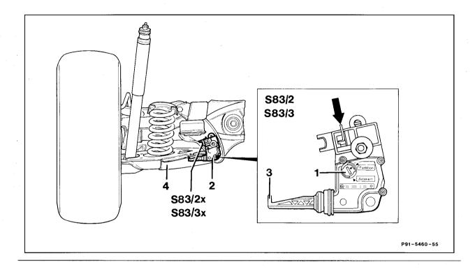
Rotary switch (1) on one of the two rear axle switches (S83/2 or S83/3) ..... turn to "Arretiert" (arrested).
