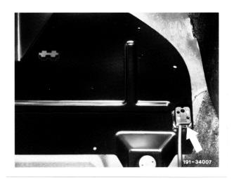
Measure insulation resistance at both occupied poles of the 4-pin test coupling (X29) to ground. Reference value: ≥ 20 kΩ EEE ∞ Reference value Reference value correct incorrect Check cable harness for damage and renew if necessary. Measure resistance of detonators. Reference value: 1.0–1.7  $\Omega$ Reference value Reference value correct incorrect End of test
