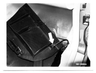
**Model 124**, 2nd version On the plate situated under the foot rest in the passenger's footwell.
