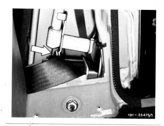
2 When the series was introduced, some vehicles were built with no colored mark on the cable of the belt tensioner. These must be tested as follows:
