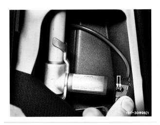
Reconnect right-hand belt tensioner detonator (R12/2).
