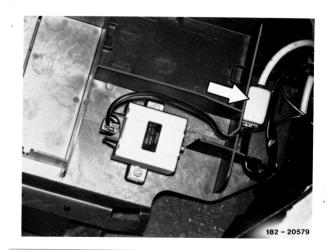
Watch the warning lamp whilst turning the steering wheel to full lock in both directions with the engine running. The warning lamp must not light up or flicker.
