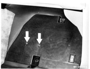
5 Disconnect red 10-pin plug connection of control unit at foot rest.
