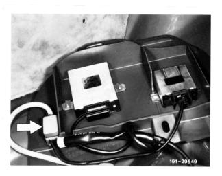
6 Disconnect plug connection and remove reserve power source.
