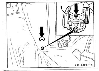
Arrow = rotation lock Seat belt inertia roller
