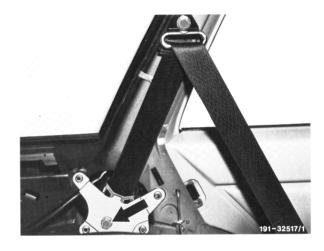
4 Unscrew screws (4 each) and remove seat belt inertia roller together with base plate.
