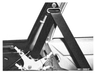
5 Unscrew screw on belt guide fitting at top.
