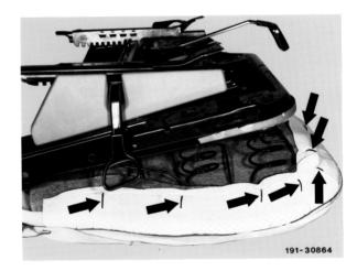
11 Unbend stapling clips on bottom of rubber hair mat and remove cover.
