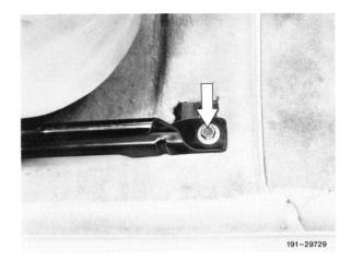
Remove screws on seat guide rails, rear.
