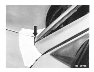
10 Align water deflector in longitudinal direction and push into plug-in clamps, starting from the rear. For this purpose, use a suitable strip of wood (approx. 150 mm long) and a rubber hammer.
