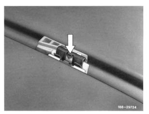
7 Install plug-in clamp with water pump pliers. For this purpose, compress holding part of plug-in clamp until an adequate preload in roof channel is attained.
