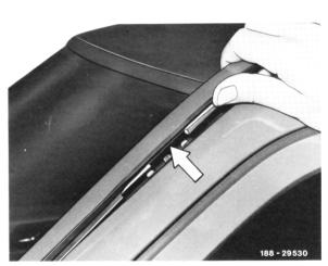
5 Mark installation position of plug-in clamps in roof channel and remove with pointed pliers.
