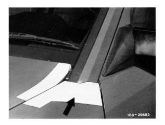
2 Push water deflector in upward direction out of 6 plug-in clamps starting at the rear.
