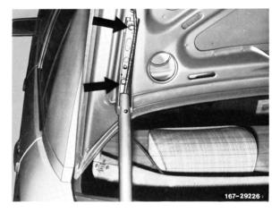
3 Loosen screws on closing eye of trunk lid.
