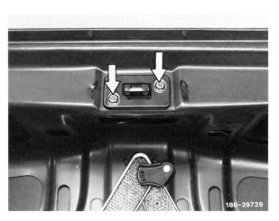
4 Adjust trunk lid in such a manner that the rear edge of the cover is flush with rear fender.
