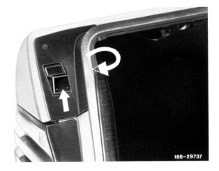
3 Loosen fastening screws of trunk lid lock and move lock in downward direction.
