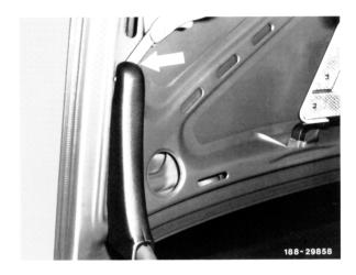
2 Loosen screws on hinge left and right.
