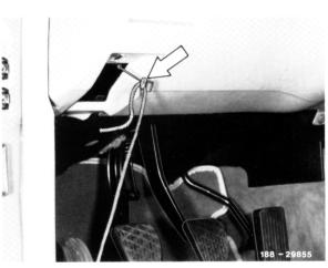
5 Force off holding bracket of rubber grommet and remove rubber grommet.
