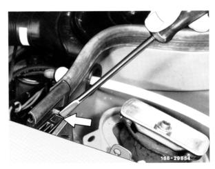
6 Remove clips of cover under engine hood lock (burglar protection), while disengaging detent through hole in radiator reinforcement.
