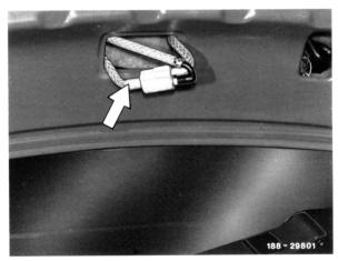
4 Pull connecting cable from righthand windshield washer nozzle.
