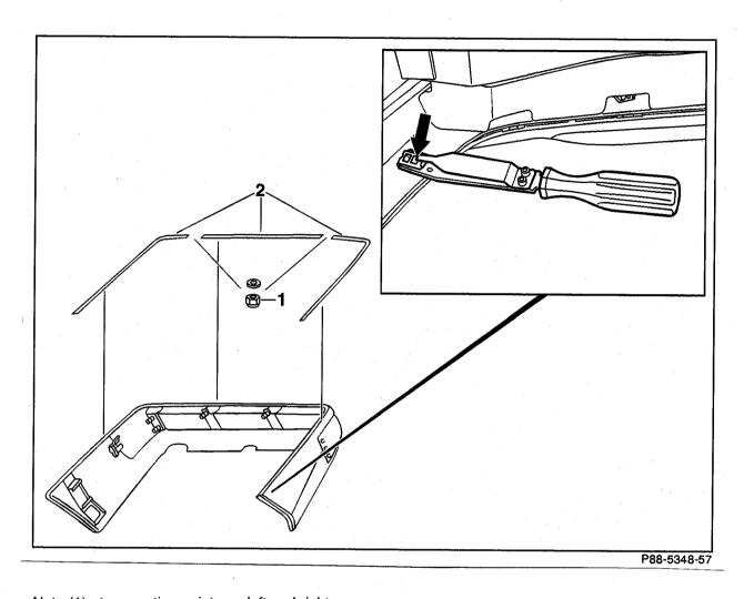
Nuts (1) at separation points on left and right ... unscrew, screw on.
