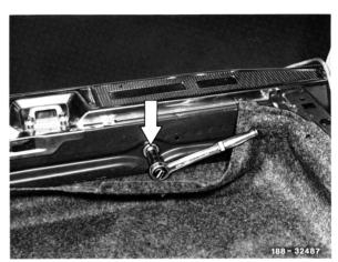
7 Check or mount seal and holder laterally on fender.
