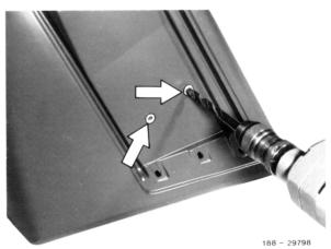
**Note**: If rivets and a riveting tool are not available, lateral holders can be screwed on.
