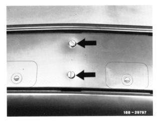
5 Drill out fastening rivets of lateral holders.
