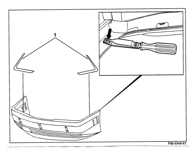
Clips (arrows, 14 each) ..... remove, install, installation tool 140 589 34 23 00.
