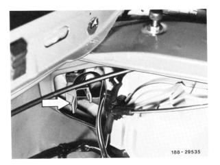
5 Remove screws in cutout of flasher lamp unit.
