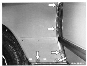
Remove screws on flange at top.
