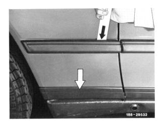
2 Remove screws on front wall pillar and on side member.
