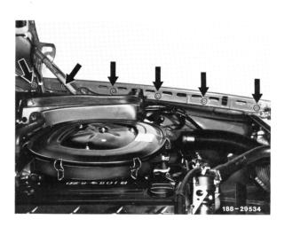
4 Push holding bracket of flasher lamp unit inwards, remove flasher lamp unit in forward direction and pull off plug connection.
