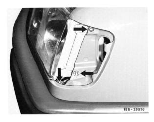
6 Unscrew screw on molding and remove molding.
