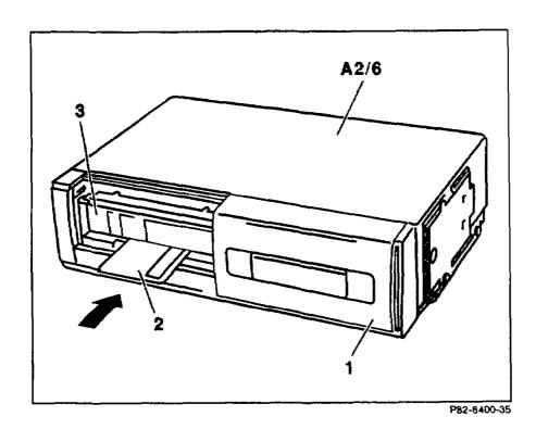
open. End cap (1) ..... insert between magazine compartment (3) and Credit card (2) or item with similar shape ...... CD player with changer (A2/6) until resistance is felt. release with slight pressure. Catch
