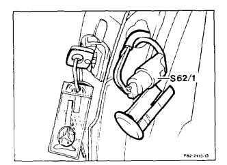
Remove plug connection (S62/1) of left-hand or right-hand door.
