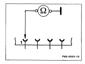
Test operation of alarm signal horn (H3) and negative cable for alarm horn for open circuit; rectify any open circuit.
