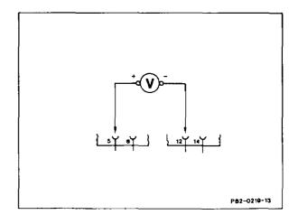
Test brown/blue cable from contact 12 up to the radio security contact for open circuit or short circuit to ground; rectify any open circuit or short circuit.
