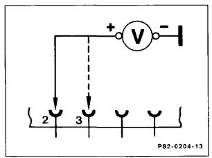
Test gray cable from contact 2 (terminal 58R) and gray/white cable from contact 3 (terminal 58L) up to fuse 3 and fuse 8, respectively, for open circuit, rectify any open circuit.
