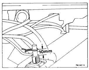
Test brown/red cable from contact 9 up to switch and the switch itself for open circuit or short circuit to ground; rectify any open circuit or short circuit.
