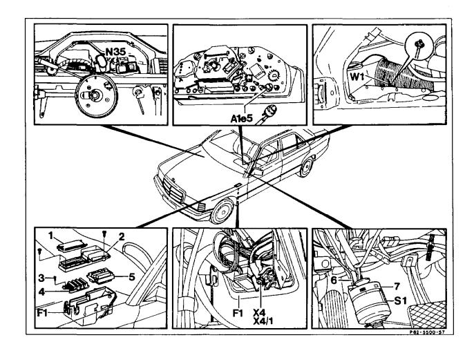
Covers (1 and 2) of fuse and relay box (F1) .... remove, install (54-1255, step 1). Phillips screw (3) ..... unscrew, screw in. raise, place back in position (step 2). Fuse carrier (4) ..... Fuse and relay box (F1) ..... press apart, release relay holder (5) and raise (step 3).
