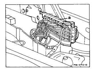
14 Run cable (grey/violet) to exterior lamp switch (S1) and press contact jack into free terminal K2 of rotary lamp switch coupling.
