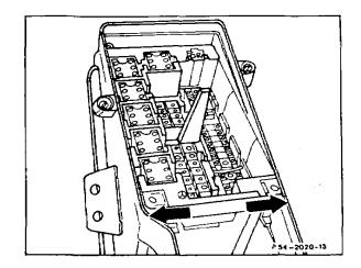
4 Screw daytime driving lamp control unit (N35) onto retaining plate in right footwell.
