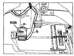
5 Lay daytime driving lamp wiring harness from right to left over heater box and secure with existing cable straps.
