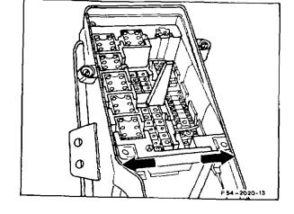
4 Screw daytime driving lamp control unit (N35) onto the holder behind the instrument cluster.
