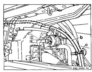
6 Connect 12-pin coupling of wiring harness to daytime driving lamp control unit (N35).
