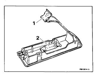
Rear dome lamp (E15/3) . . . . . . release, snap in (arrow).
