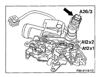
Door lock on tailgate ...... Tailgate infrared remote control (IFZ) receiver unit (A26/3) .....
