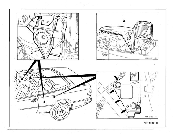
Loudspeaker bracket (2) remove, install.
