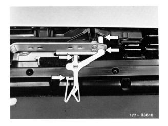
**Note**: The two rear fastening screws have metric threads. To make sure that the tilting/sliding sun roof frame centers itself in relation to tilting/sliding sun roof cutout, tighten the two front fastening screws at left and right first.
