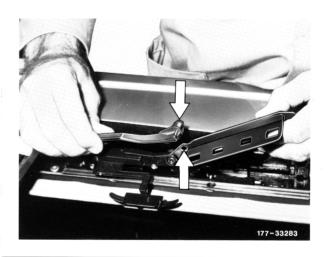
5 Slide angular lifting arm up to stop in forward direction, tilt upwards and remove at an angle in inward direction.
