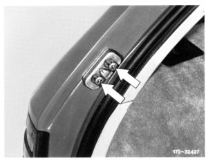
**Note**: If tailgate binds on lock, adjust by removing or inserting a spacing washer at lock strap to adjust distance in relation to lock.
