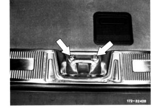
7 Tighten screws on stop of rear pillar and on strap for tailgate lock.
