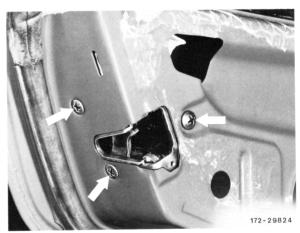
**Note**: When opening grab handle, make sure that the grab handle is at rest behind actuating lever of door lock.
