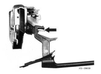
8 First tighten the two fastening screws on face side, then those on door inside panel to 8 Nm.
