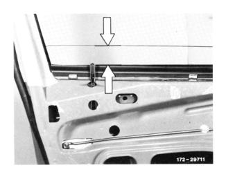
4 Unscrew nut on window lifting rail at front and disconnect window lift arm.
