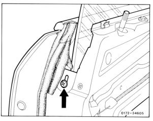
6 Unscrew guide shoes at front and rear and remove.
