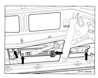
5 Loosen screw on guide wedge.
