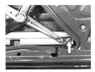
5 Lift window at the rear and extend slide shoes at cutout of window lifting rail.
