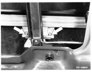
8 Extend guide member out of window lifting rail.
