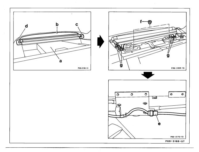
Covers (b, c, d) ...... unclip, clip in. Rear shelf (a) ..... remove, install (68-458). Mounting nuts (f) ...... screw off, screw on (6.5-7 Nm). Plug connector on motor (e) ...... disconnect, connect. remove, install.
