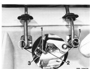
6 Knock out headrest uniformly toward the rear out of bearings, by means of light blows with ball of thumb and remove.
