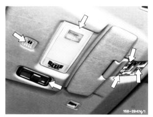
5 Push complete roof operating unit toward the right and out of trim by means of plastic wedge. Pull off plug, remove roof operating unit (2nd version).
