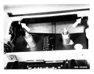
23 Insert adjusting screw on connecting linkage of fresh air flap and adjust in such a manner that the flap is closing under a light preload.
