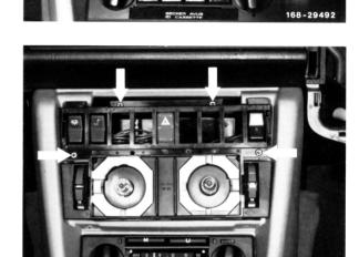
14 Pull off switch for heatable back window, push switch carrier at the right forward out of detent and remove at the left toward the rear.
