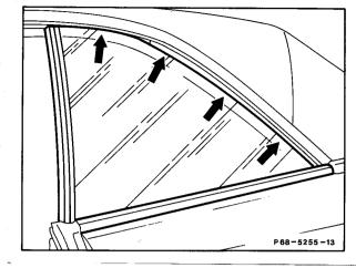
16 Check tilt of side window and ensure that side window is parallel in side window shaft, adjust, if required. For this purpose remove panelling on rear fender (88–800 Section B) and rubber grommet.
