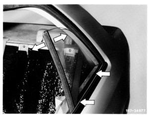
13 Loosen nuts and adjust side window by turning adjusting screws (WAF 5.5) in such a manner that it will run in parallel out of window shaft into sealing strip.
