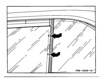
26 Check position of rear side window in relation to window in driver's door, adjust, if required.
