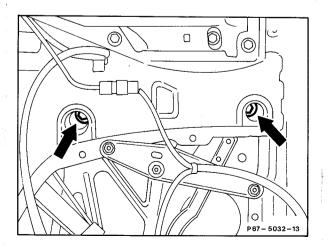
9 Continue to open rear side window until the third screw (arrow) on the window lifting rail is also visible. Then loosen screw.
