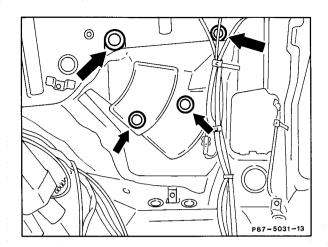
5 Preliminarily adjust top stop with screws (arrows) so that approx. 2 mm of the oblong hole is visible above the screw head (basic adjustment).
