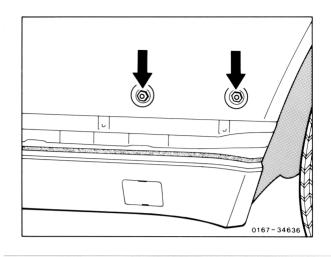
Additional possible adjustments of window tilt at upper mounting nuts of window lift
