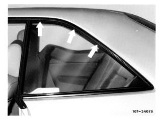
12 Check tilt of side window and parallel location in window shaft and adjust, if required. For this purpose, remove panelling on rear fender (88-800) and remove rubber grommet.
