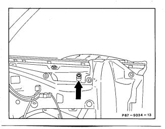
14 Adjust height of rear side window so that the top edge of the glass contacts the sealing profile with slight tension when the side window is closed.
