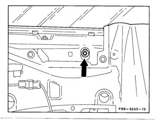
30 Loosen screw (arrow) on bottom stop after removing plastic cover (1). When installing seal all the way around with window sealant, part no. 001 989 31 20.
