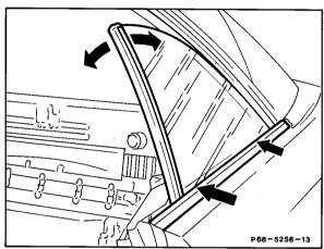
17 Loosen nut and adjust side window by turning adjustment screw (WAF 5.5) so that it runs out of the window shaft and into the sealing profile parallel.
