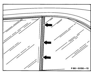
13 Loosen screw on top stop.
