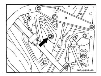
10 Adjust rear side window in longitudinal direction so that the rear edge of the window in the driver's door is located in the center of the groove (arrow) in the sealing profile on the rear side window when the windows are closed.
