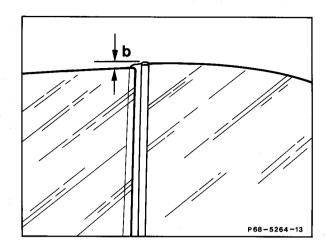
Correction is possible by moving top stop slightly.
