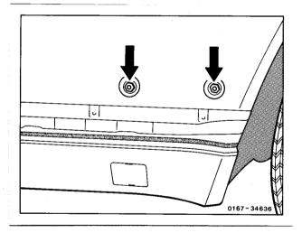
Additional adjustment possibility for window tilt on top mounting nuts for window lift.
