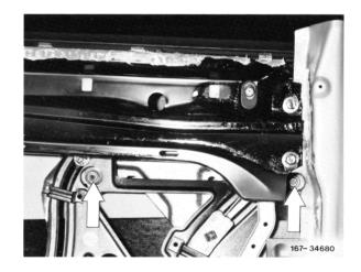
6 Adjust rear side window in longitudinal direction in such a manner that with windows closed, the window pane of the driver's door is resting in center of sealing strip groove.
