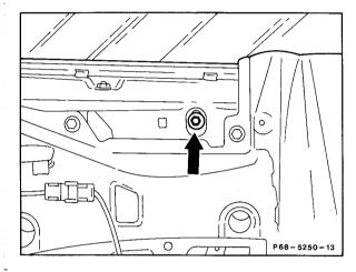
6 Loosen nuts (arrows) on top window lift and preliminarily set window lift to center of oblong holes (basic adjustment).
