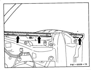
3 Remove rear loudspeaker together with bracket (2).
