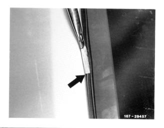
6 Push trimstrip outwards starting from below up to upper edge with drift. Then force trimstrip at top from connecting link toward corner in upward direction from pane.
