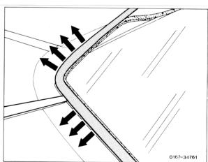
**Note:** If trimstrip is stuck, apply counterhold with plastic wedge so that the trimstrip will not be twisted.
