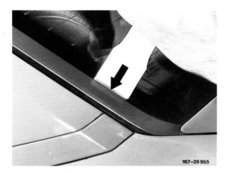
**Note**: If a trimstrip is stuck, apply counterhold with plastic wedge so that the trimstrip cannot twist.
