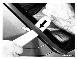
7 Pull out trimstrip at top starting from center. Remove link (arrow) on respective trimstrip half prior to pulling out.
