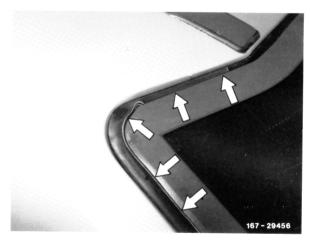
5 Push rubber cover on trimstrip aside and apply soap water all-around between rubber and body.
