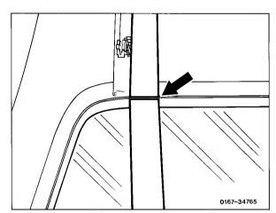
**Note:** To permit displacement of windshield glass during alignment, mask holding strip with adhesive tape.
