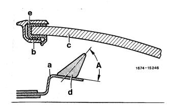
34 Place on lower rubber pads (item 30) and align according to adhesive tape strip at top. Place on adhesive bead and push into holding strips.
