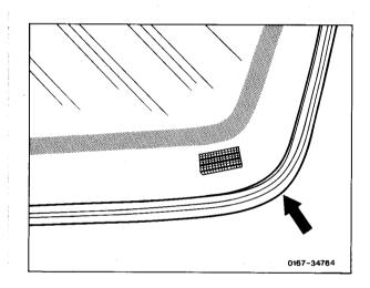
23 Coat holding groove in trimstrip with soap solution and press trimstrip on pane starting at upper corner.
