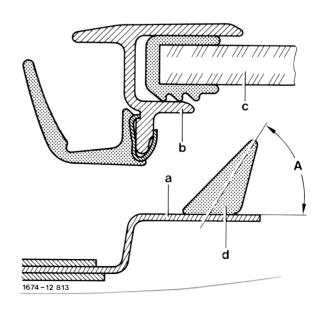
43 Place pane on lower rubber pads, align, place on glue bead and push down all-around until the trimstrip is flush with body.
