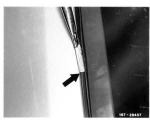
20 Starting from below, push trimstrip with punch outwards up to upper corner. Then push trimstrip at top from connecting link toward corner in upward direction away from glass pane.
