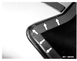
19 Push rubber cover on trimstrip aside and apply soap solution all-around between rubber and body.
