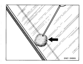
29 Renew holding strips (4 each) on body top which may have suffered damage.
