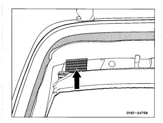
30 Insert rubber pads 10x20x13 from repair pack into glass cutout, below (arrow).
