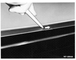
17 Push glass pane in upper range carefully in outward direction and slip plastic wedges inbetween glass and glue flange.
