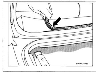
33 Remove cartridge with glue from repair pack, cut through diaphragm, remove cartridge bottom and dump chemicals. Screw on application nozzle and insert cartridge in processing gun.
