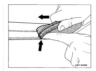
32 Check molded rubber strip in pane cutout below, renew rubber, if damaged.
