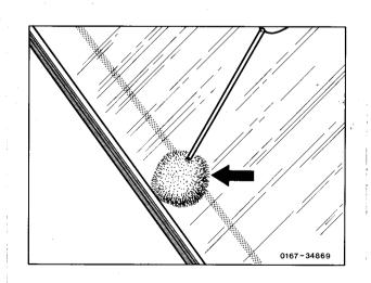
41 Insert rubber pads 10x20x13 from repair pack into pane cutout, below.
