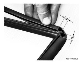
34 Coat holding groove in trimstrip with soap water and push trimstrip on pane, starting at upper corner.
