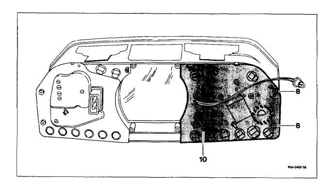
Screws (8) ..... unscrew, screw in. Gauges (10) ..... remove, insert.
