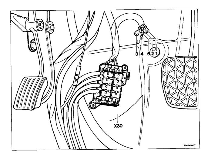
Arrangement of plug connection of optional equipment block (X30) in front left footwell.
