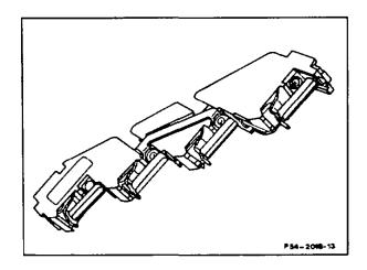
As of 07/86 vehicles with automatic climate control are fitted with an auxiliary fuse box (F15), automatic climate control (KLA)/automatic temperature control (TAU) blower motor, with a 30 A leaf fuse for the blower motor.
