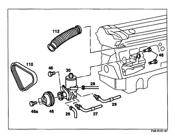
Air intake hose (112) . . . . . . . . . . . Remove, install.
