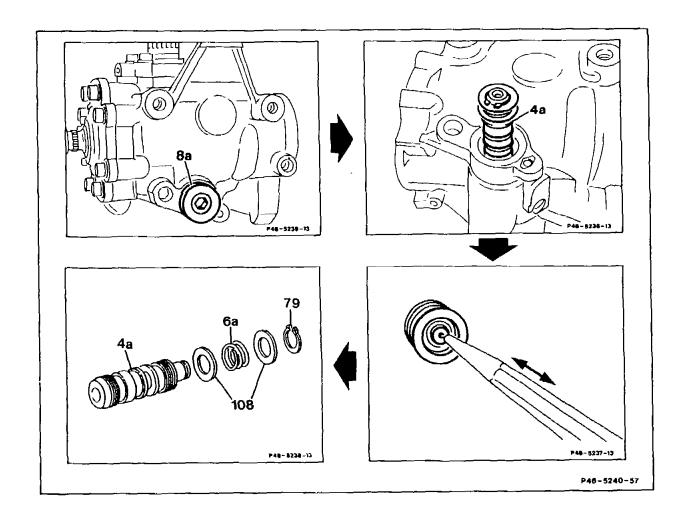
unscrew, screw in, 100 Nm, replace seal. remove, install at steering gear.
