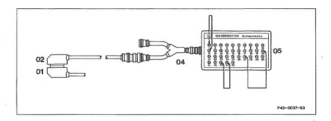
Bridges to socket box (example test step 1)
