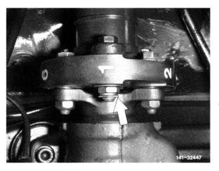
8 Repeat this procedure on all 6 fastening screws, while mounting the balancing nut (arrow) or balancing washer on each of the nearest hexagon bolts. Write down the obtained respective results.
