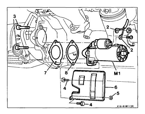
Battery ground cable ..... disconnect, connect. Steering ...... turn to left. Shield on pitman arm ...... remove, reinstall. Bolts (4) ..... screw out, screw in. screw off, screw on. remove, install. Electrical connections (2) ...... disconnect, reconnect. screw out, screw in. Starter (M1) ...... remove downward, install from below, remove and reinstall shim(s) (8) and splash guard (7), if present.
