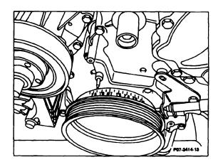
2. Loosen mounting bolts (arrows) at injection pump flange and bracket (arrow).
