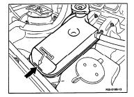
Check concentration of antifreeze/anti-corrosion protection. Top up only on separate order.
