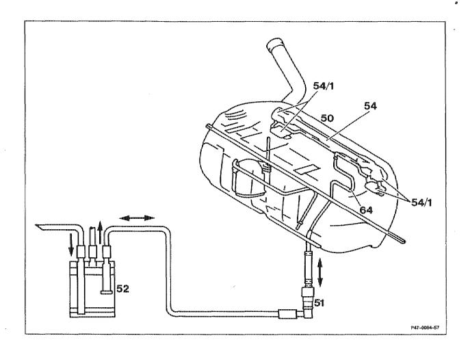
The vent system consists of a central pipe (54) with interruption vessels (54/1) at the ends. The interruption vessels (54/1) prevent the fuel escaping along the vent pipe (64). The vent pipe runs from the central pipe (64) through the vent valve (51) to the activated charcoal filter (52).
