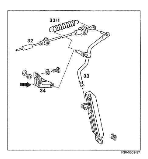
Footwell trim remove, install. Return spring (33/1) ...... detach, attach. Bowden cable (32) at accelerator pedal lever detach, fit on. Bolts of firewall pivot bearing ..... unscrew, screw in. Firewall pivot bearing (34) together with accelerator pedal lever (33) ...... take off, fit on.
