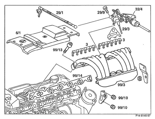
Connecting rod (29/1) to vacuum control flap at accelerator control linkage ..... de
